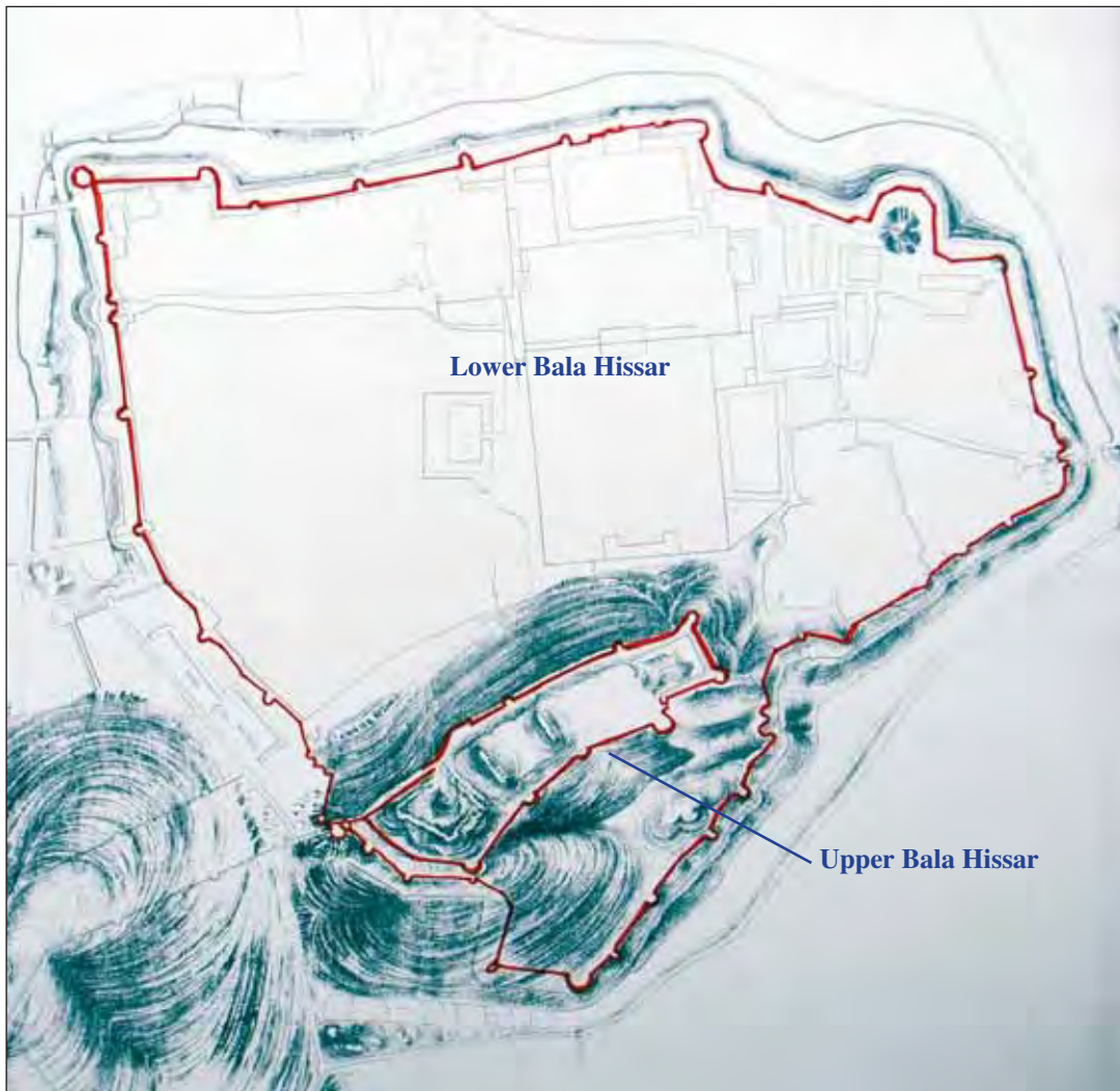
Figure 2. A sketch plan of the Bala Hissar in 1839. The fort had two parts, the Bala Hissar Bala , or Upper Bala Hissar, which was sited on a small hill and also called the citadel or Arg , and the Bala Hissar Payin , or Lower Bala Hissar, which contained palace buildings and a small township. The whole was rather like a large “motte and bailey” castle. [Adapted from plan in Figure 5.]
