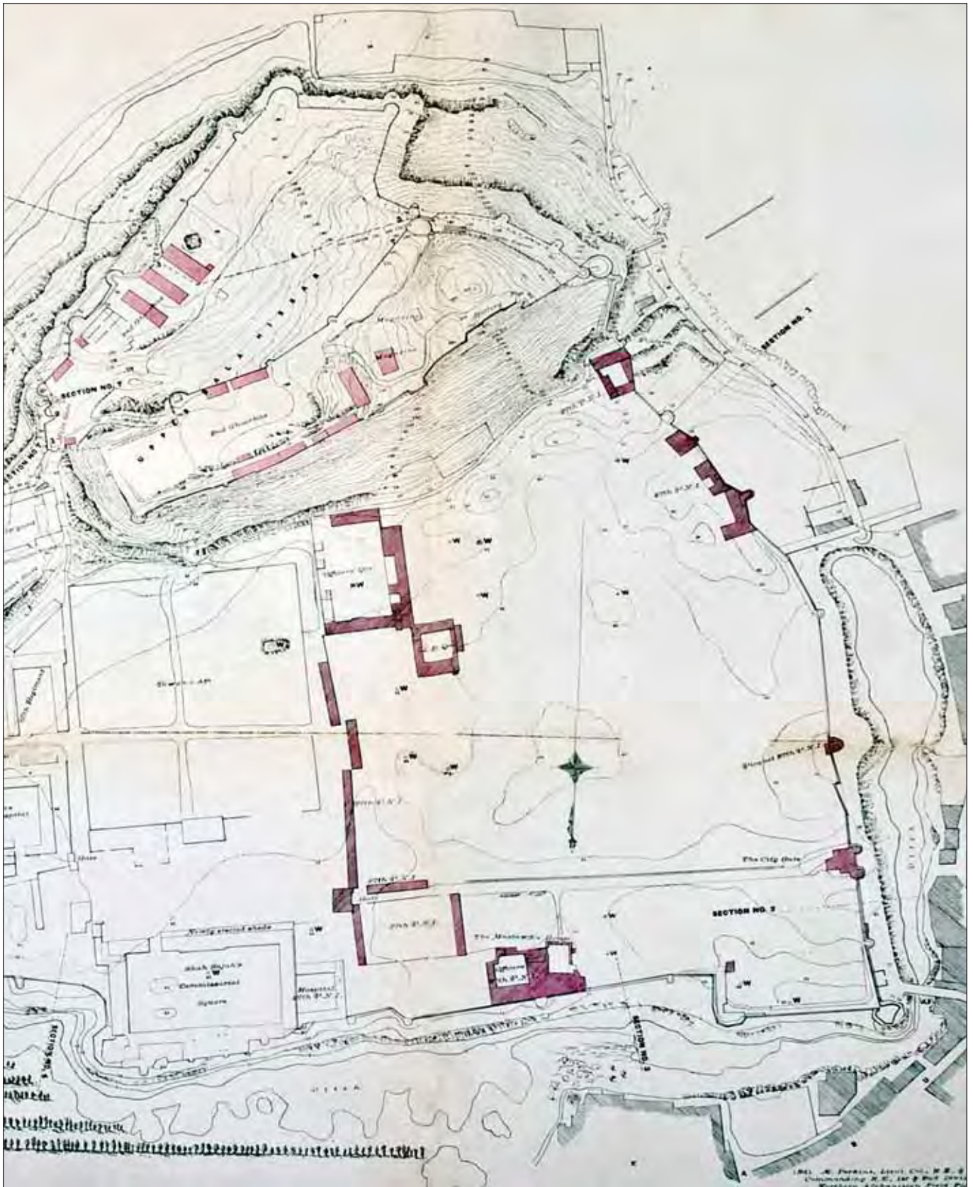
Figure 44. Part of “Cabul Defences No. 6. Plan of Bala Hissar, Subsequent to Demolition and Reconstruction.” Surveyed by Lieutenant J. Burn-Murdoch, RE, 1880. Note: South is at the top . Buildings marked in light red were new accommodation for troops, those in dark red were structures strengthened as part of the defences against an attack from the direction of the city. The plan shows that the housing in the western sector of the fort had been cleared. The nearest buildings of the city are shown hatched on the bottom-right of the plan. [Institution of RE]
