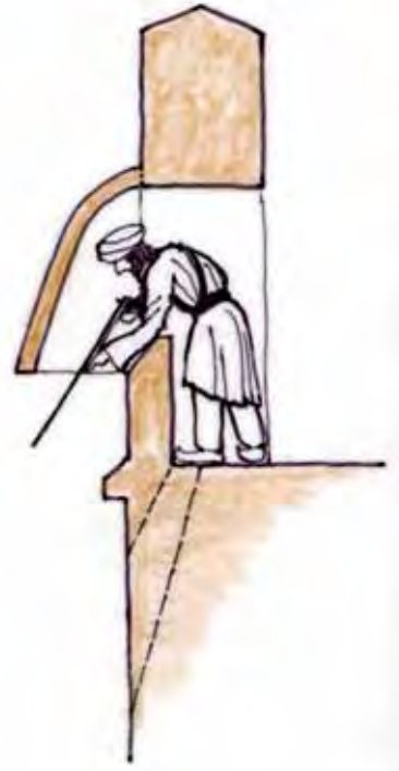
Figure 8. Sketch showing hooded (or projecting) firing-points. [Ian Templeton.]
